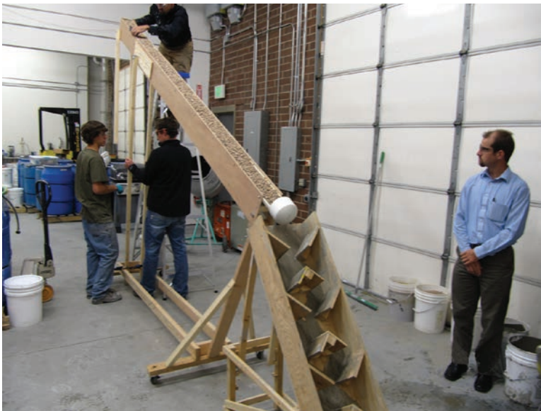
Preparing to mix pea gravel and tailings slurry using a relatively continuous feed apparatus at the Paterson & Cooke Facility in Golden, CO.
