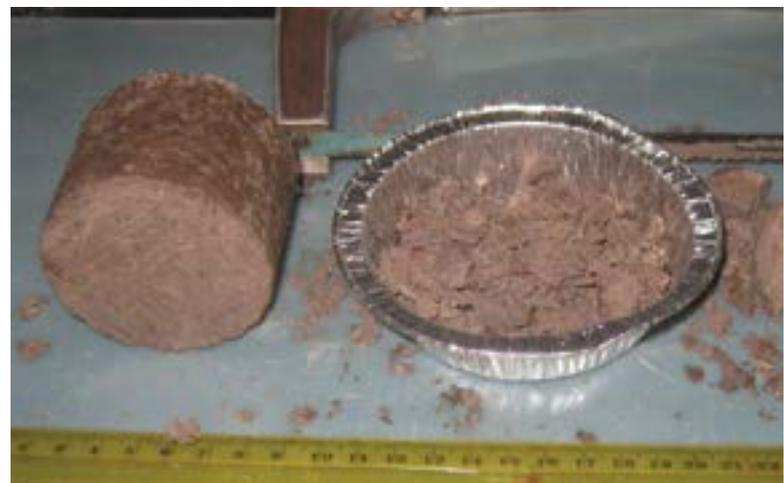
to measure the moisture content (Fig. 9). The resultant densities of 1.72 to 1.84 t/m<sup>3</sup> (107 to 114 lbs/cu ft) indicated that 1.8 t/m<sup>3</sup> (112 lbs/cu ft) should be appropriate for estimation of in-situ ‘wet’ bentonite resources in the 5D bed at the Australian mine (Table 4).
