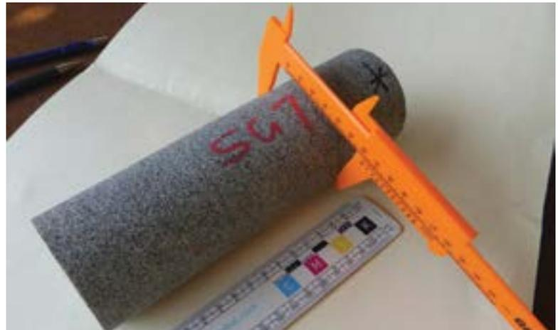
The caliper method yielded comparable results to the Archimedes method (uncoated, vacuum packed and paraffin wax). However, the ‘cling wrap’ method proved to be unreliable as it entrained air (reducing the density) and was not completely waterproof.
