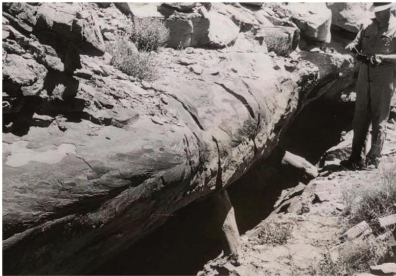
Perspective view of the inner (concave) surface of a mined roll at the Cougar Mine. This view shows the form of a typical C-shaped roll.
